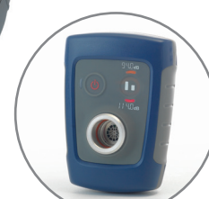
CEL-120 Calibrator Compatible with dBadge2 & SLMs
